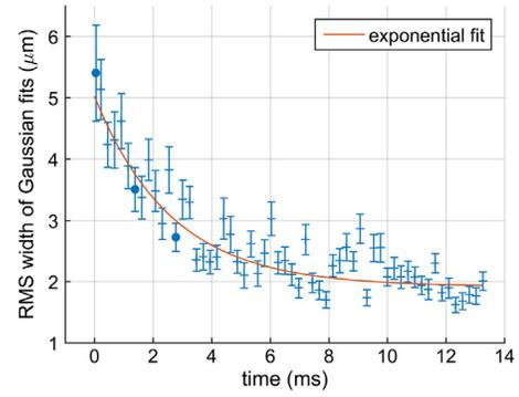
FIG. 3. Spread of the resonance fluorescence of an ion in the axial direction expressed as rms width  $\sigma$  of the fitted Gaussians (some of which are shown in Fig. 2, the corresponding points are marked with filled circles) depending on time. An exponential fit is shown in red.
