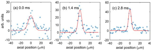
FIG. 2. Ion images summed over the radial direction (blue crosses) and Gaussian fits (red solid lines) at (a)  $t = 0$  ms, (b)  $t = 1.4$  ms, and (c)  $t = 2.8$  ms after opening the cooling laser. The heating time  $T_H$  is 15 s, exposure time is 0.2 ms, 209 experimental runs are summed.
