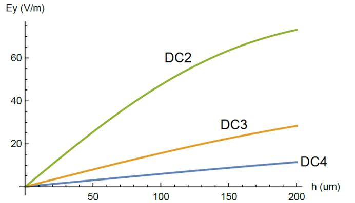
FIG. 2. Axial component of the electric field at the trapping position,  $E_y$ , created by 1 V voltage applied to electrodes DC2, DC3 and DC4 vs. trapping height  $h$ . DC1, RF and DC0 create electric fields with zero y-component.
